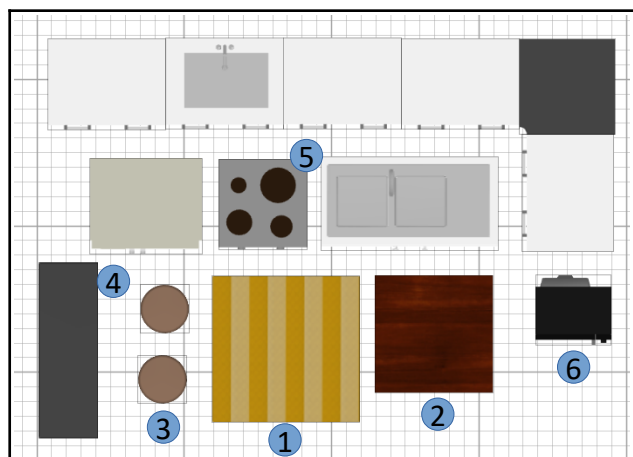
1- Table 100x100 2- Table 80x80 3- Tabourets 4- Plan de travail 120x40 5- Gazinière 6- four micro onde
