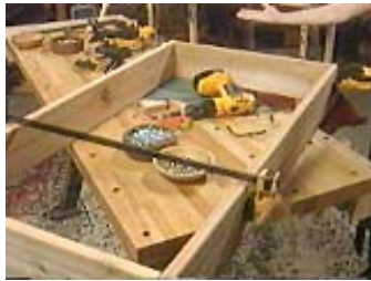
Clamp the apron or skirt frame together
