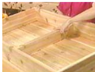
Use a center brace to help support the table top
