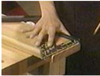
Check the end of the board for squareness and splits
