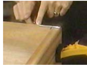
Choose screws that are long enough to have at least half their length in each pieces
