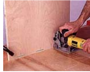
3--Use a plate joiner to make the slots for the case. Clamp case sides vertically and register the slots against your work surface.
