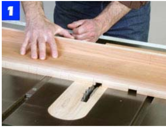
After cutting the 1 x 8 lattice stock to length, lay out the half-lap joint notches and cut them with a dado blade.
