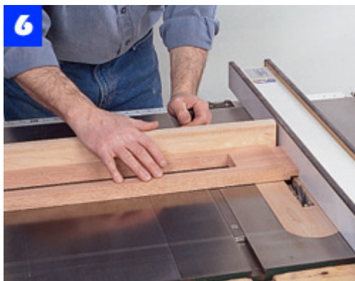
Use a dado blade to cut the tenons on the apron ends. The rip fence acts as a stop to ensure uniform tenon length.
