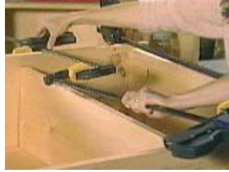
Use two clamps together if one is not long enough
