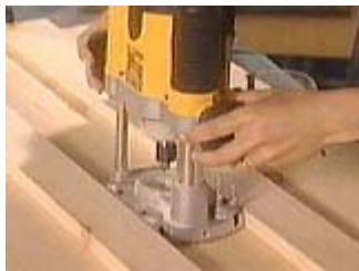
Set up a guide fence on either side of the router for the 'V' groove
