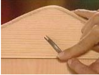
Carving on the top trim with a 'v' carving tool
