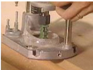
Plunge router with beading bit
