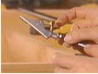
For blind nailing, use a tiny plane
