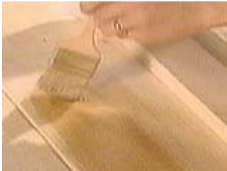
Apply a water based aniline stain with a brush
