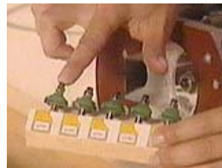
Choose a bit for the trim and rout an edge on the bottom trim piece
