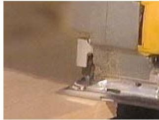
Cut out the shape with a jig saw and scrolling blade
