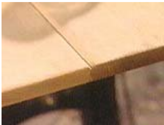
For less color on end grain (left) spray with water first
