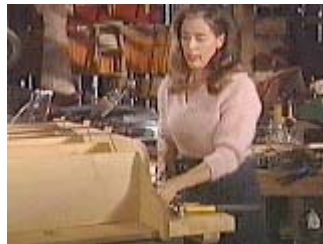
Shelves squared, clamped and ready for nailing
