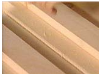
Test for depth and rout a groove along each joint on the back
