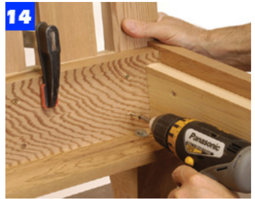
Temporarily clamp the chair back to the base and fasten the parts with galvanized deck screws.
