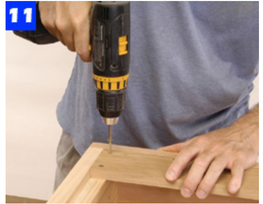
11 Screw the foot rails to the cleats. Note that the back edge of the rear chair foot rail is beveled to fit the back rail.
