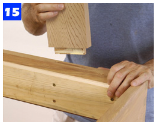
Spread glue in the side-rail mortises and on arm-post tenons. Join the parts and clamp to pull the joints tight.
