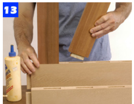
13 Glue the chair back slats to the back rails. When the glue is dry, apply glue and add the back stiles.
