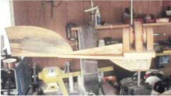
Almost ready—the wooden frame and tail are attached.
