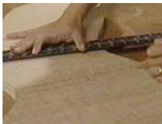
Mark out a centre slot three quarter inches wide and half way from top to bottom
