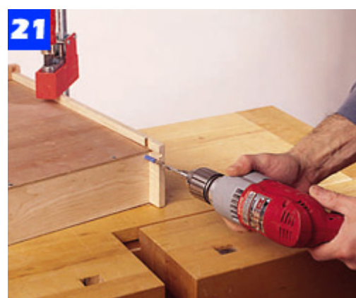
Use masking tape on a drill bit to mark a hole's depth, then bore the stopped holes in the back of each drawer.
