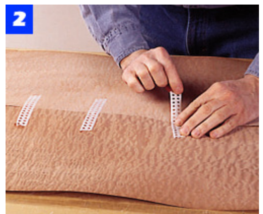
Make the edges of two book-matched veneers perfectly straight and smooth, then join the sheets with veneer tape.
