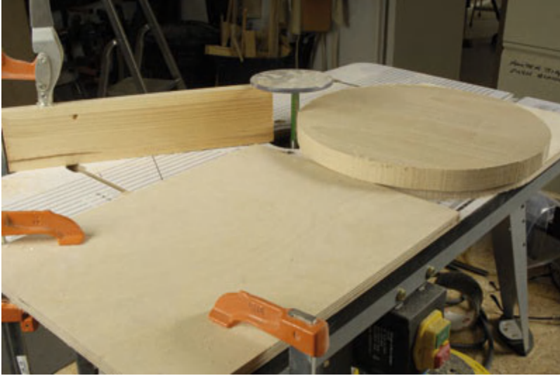
12 The jig setup ready to cut; note the stop board clamped firmly in place and the cutter guard
