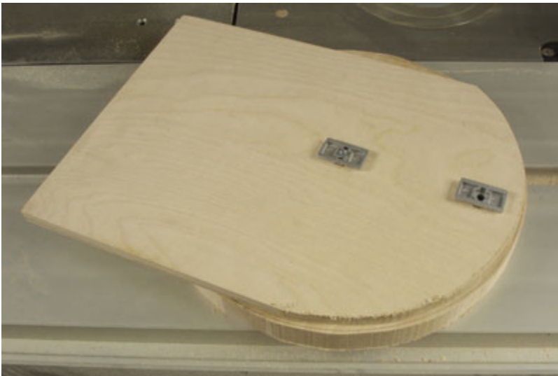
11 The underside of the sliding circle-cutting jig with a blank attached
