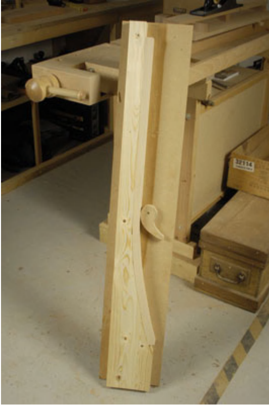
6 The jig is turned over in order to thickness the other leg edges
