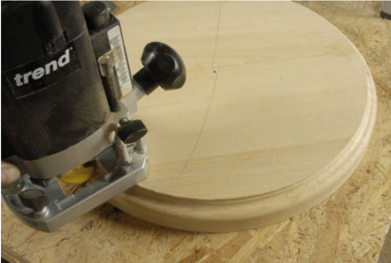
14 Machining the underside of the top using a large classical profile cutter
