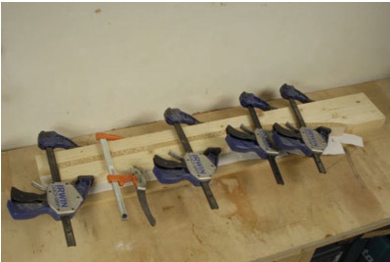
4 These clamps are immensely powerful but the rubber pads prevent damage to the workpiece
