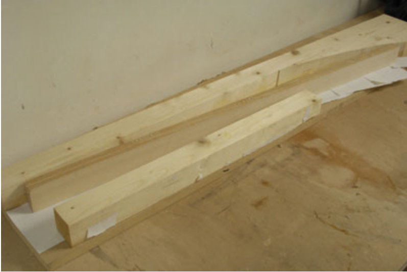
3 The jig with the glued components ready to be clamped in place
