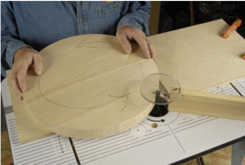
13 When cutting hold the blank firmly to prevent it spinning the wrong way and causing damage; note the rotation marks as a clear reminder to the operator
