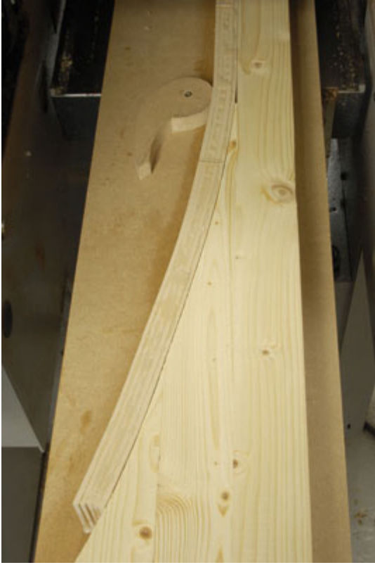
5 The clamps are replaced by an MDF cam for thickening
