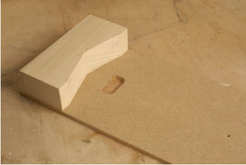
18 The underside of the mortising jig showing the bandsawn detent which allows the jig to sit properly on the curve
