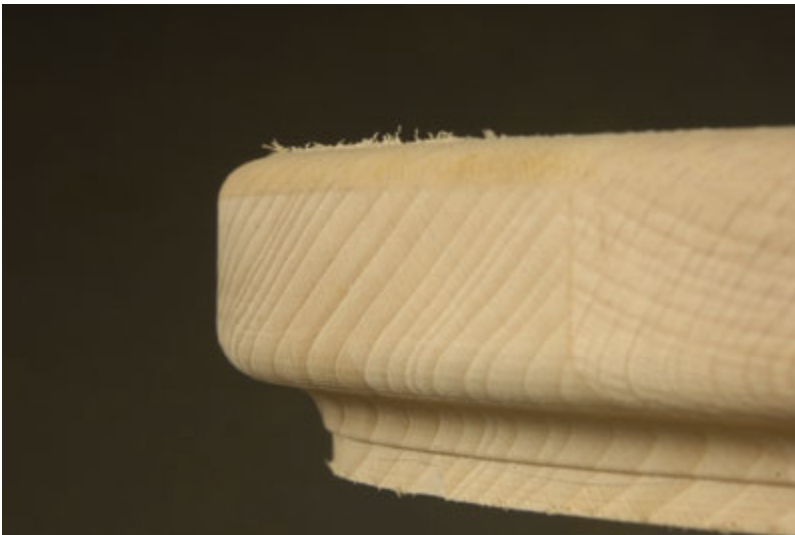
15 The resultant shape after doing both top and bottom cuts before sanding; note the slight step near the bottom of the profile
