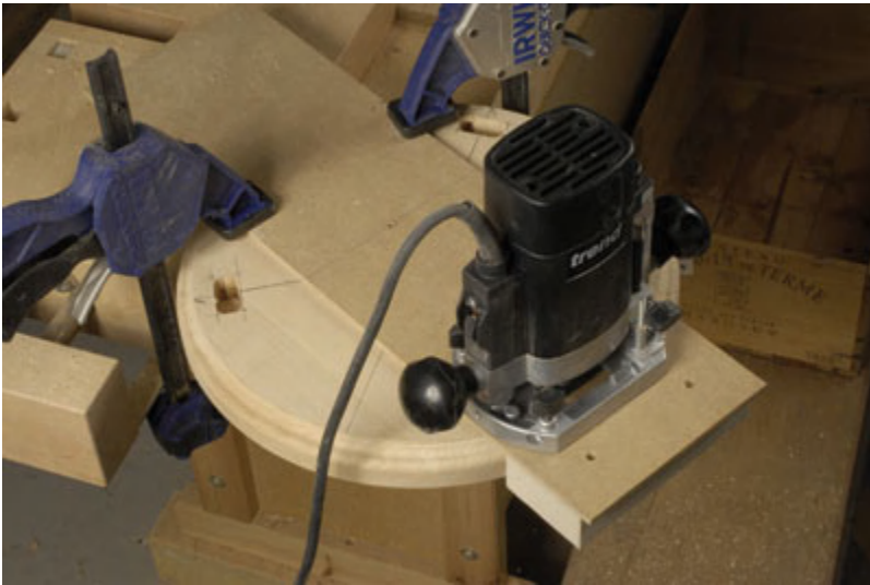
19 The jig firmly clamped in place and overhanging the bench for mortising
