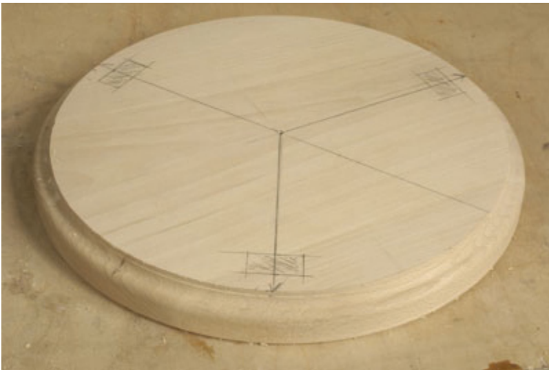
17 The "pie-chart" lines set out to allow marking the mortise positions
