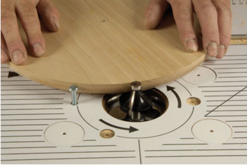
16 Machining the large roundover on the lower platform is safer done on the router table; note the improvised lead-in pin
