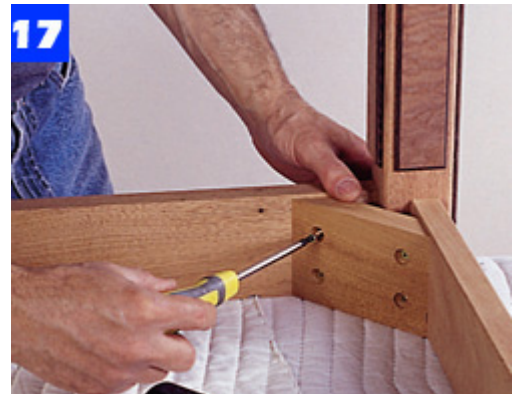
Cut corner blocks to size with 45° angles at each end. Countersink screwholes in the blocks and secure to the aprons.
