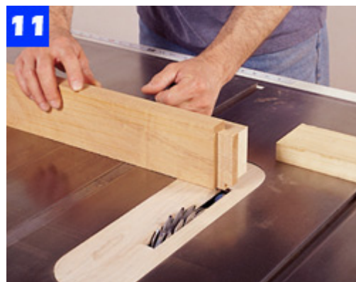
Use a dado blade in the table saw to cut the apron tenons. Clamp a stopblock to the table to ensure uniform cuts.
