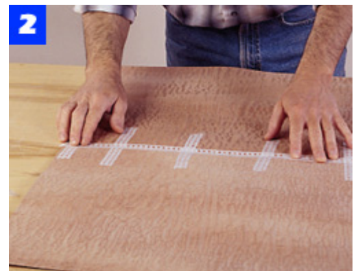
Join adjacent sheets of veneer with lengths of veneer tape across seam. Add tape along seam to hold joint tight.
