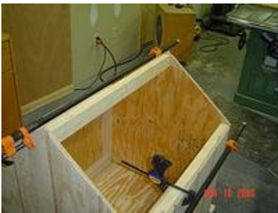
Figure 1. Temporarily attaching ridge pole.
