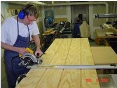
Figure 1. Cutting front/rear panels to rough length.
