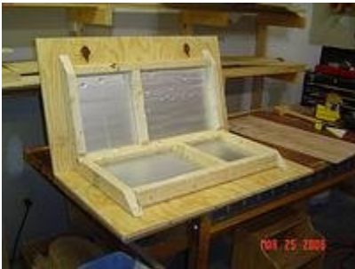
Figure 7. Underside of roof with insulation panels in place.
