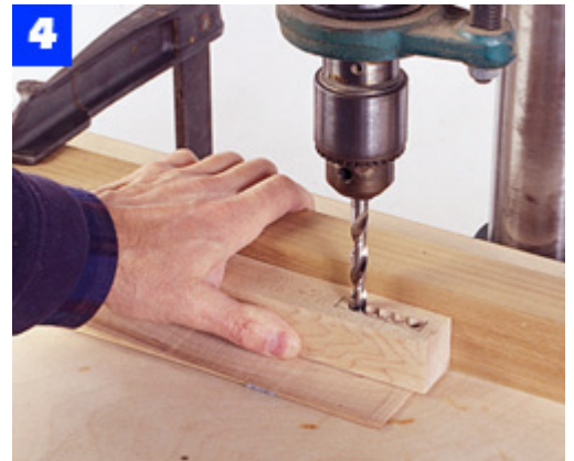
Begin the upper back rail mortises by boring a series of 3/8-in.-dia. holes. Then finish the job with a sharp chisel.
