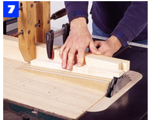
Construct a jig for cutting the angled side-rail tenons on your table saw. The ramp holds the rails at a 4° angle.
