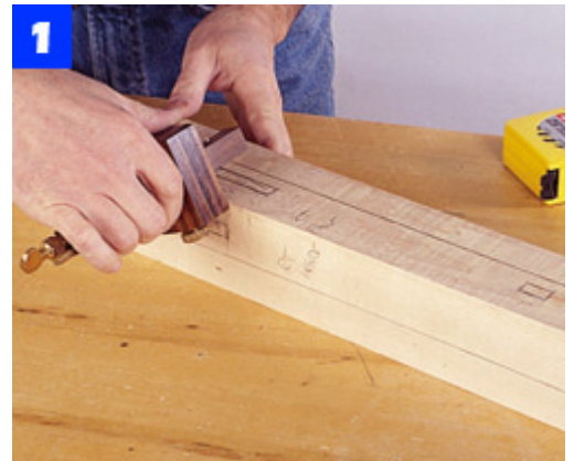
Use a tape measure, square and mortise gauge to lay out the locations of the mortises in the leg blanks.
