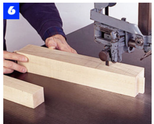
Band saw the curved shape of the rear rails. Finish the rails by smoothing with a spokeshave and scraper.
