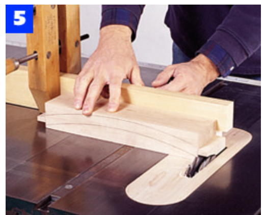
Use a dado blade to cut the tenons on the curved rail blanks. The blade height is different for front and rear faces.
