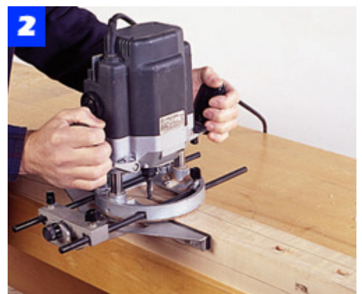
Rout the mortises with spiral up-cutting bit and edge guide. Take two or three passes to avoid overloading the router.
