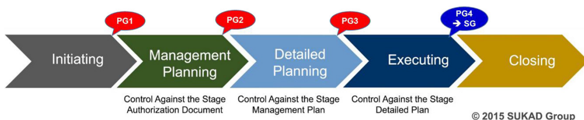
Figure 12: Stage Control and Control Reference Points
