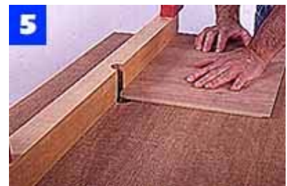
Mount a straight bit in the router table and cut the rabbets on the back sides of the side and door panels. Then sand the panels.
