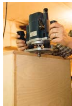
Go slowly while rounding over the edges, as the cherry can tear out and splinter if a cut is rushed. The roundover is key to the smooth, clean feel of the piece.
