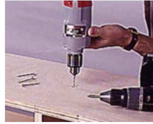
6--Bore and countersink pilot holes into the top of the short partitions. Then drive screws to fasten the partitions and panel.
