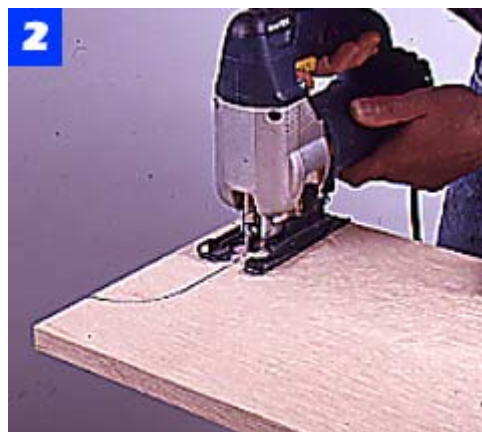
Cut and joint stock for the sides, top, bottom, partition and shelves. Then cut slots in mating edges with a plate joiner.
