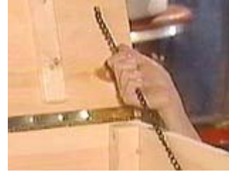
Choose a chain that is strong enough for the weight of the lid.
