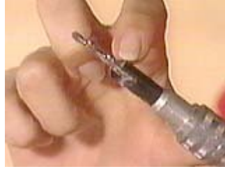
Use a counter sink bit to allow the head of the screw to set deep enough for a plug.
