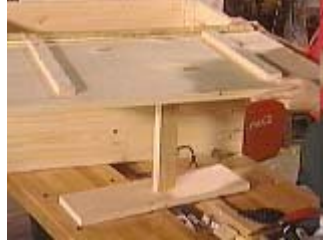
Use the jig to help hold up the lid while attaching the hinge.
