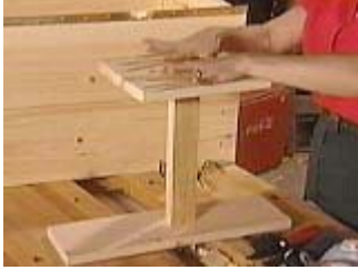
Make a jig to help hold the lid while attaching the hinge.
