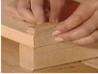
Make a jig to help locate the screws evenly.
