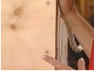
Use wooden plugs to cover the screw heads.
