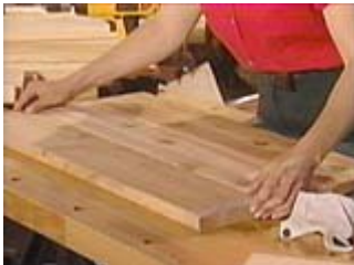
Three one inch thick cedar decking boards make the bottom of the chest.
