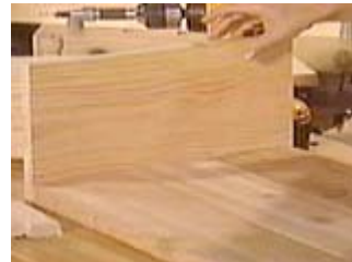
Cut the length of the side boards to match the width of the three bottom ones.
