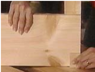
Make a new jig for the front so that the screws go into the corner posts.
