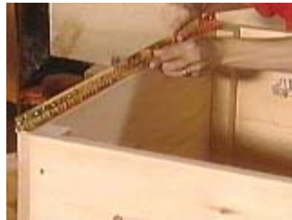
Attach the piano hinge to the box first.
