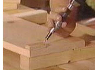
Use the jig to locate the position of the screw for drilling.
