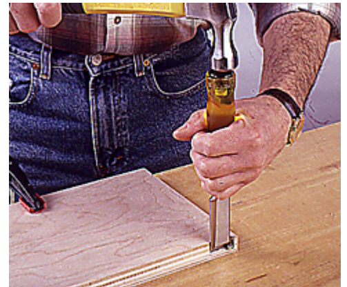
13--Cut a stopped rabbet in each side of the storage shelf. Then use a chisel to cut the end of the rabbet square.
