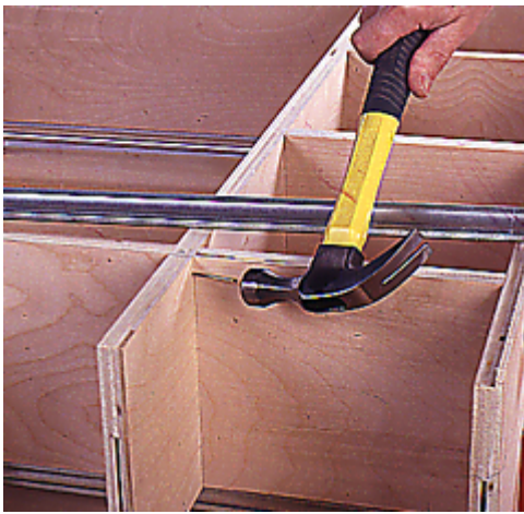
16--While holding the parts in position with clamps, drive a nail through the shelf and into the top of the inner side.
