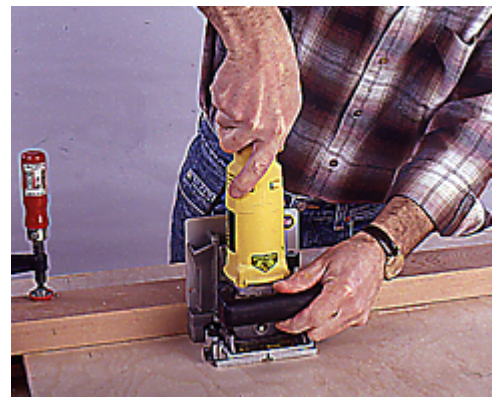
5--To cut plate slots in the panel's center, clamp a fence across the panel to guide the vertically positioned plate joiner.
