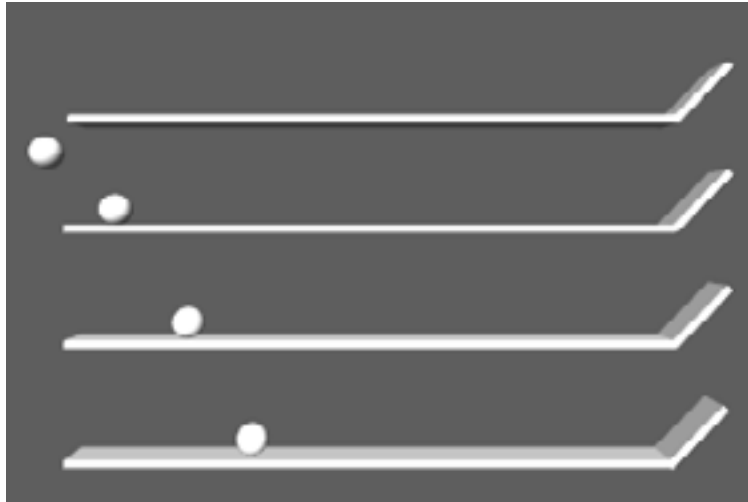
Illustration 46: The effect of the drag on the movement of the objects: upper balls have lower drag values
