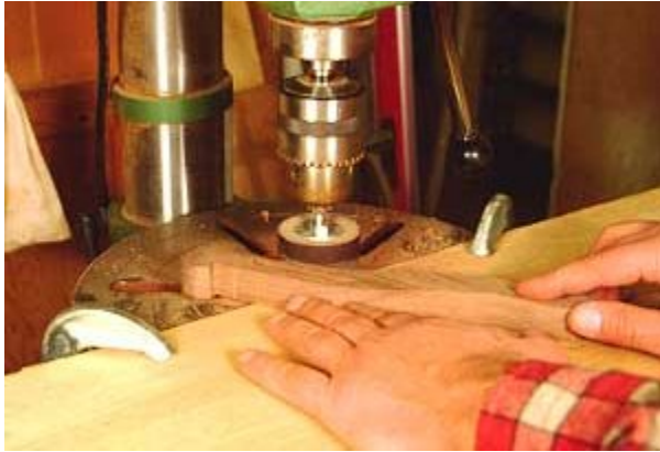
Photo 7- Smoothing the leg edges with a drum sander in the drill press.
