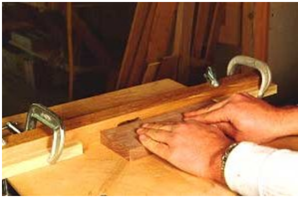
Photo 2- Next push the part along between the stops.
