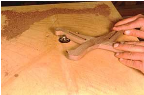
Photo 15- Round over the outsides of the legs at the router table.
