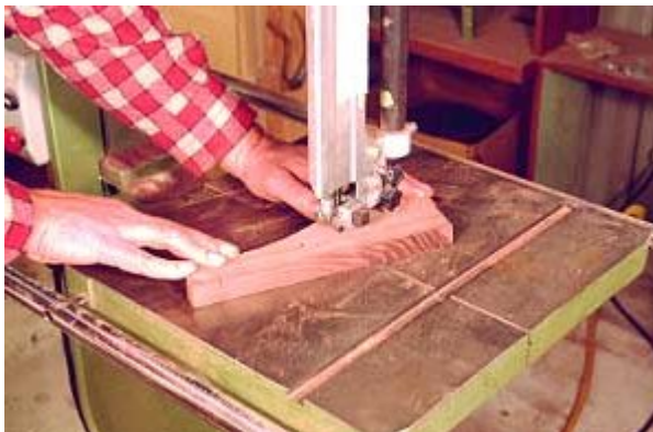
Photo 6- Cut out the legs on the band saw.
