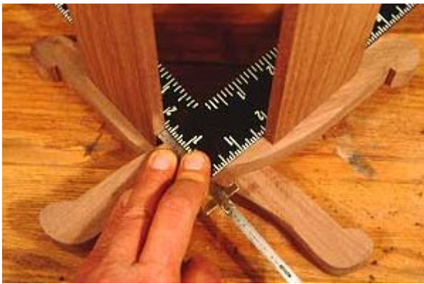
Photo 10- Aligning the parts for marking out the lap joints.
