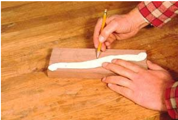
Photo 5- Make a pattern from the drawing and use it to trace the legs.
