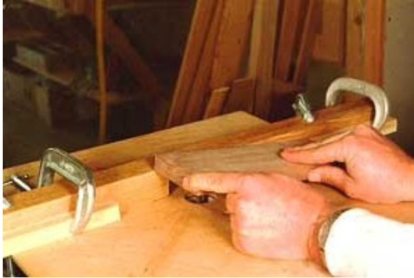
Photo 1- Lower the piece onto the bit at the router table to start the cut.
