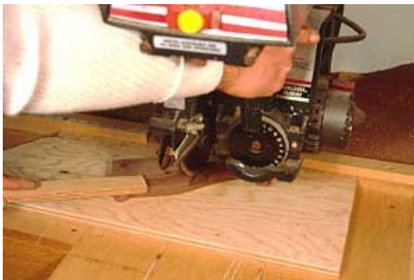
Photo 12- Use a stick to hold the part down during the cut, not your fingers, because your fingers would be too close to the blade for safety.
