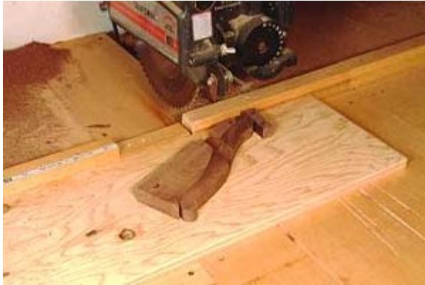
Photo 11- Radial arm saw jig for cutting out the lap joints.
