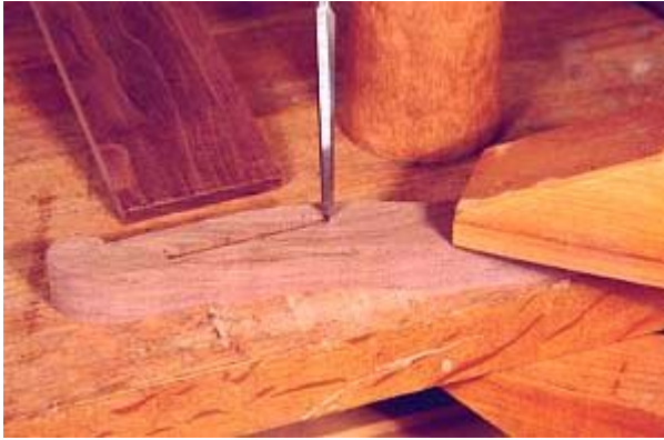
Photo 9- Square up the ends of the slots with a chisel.
