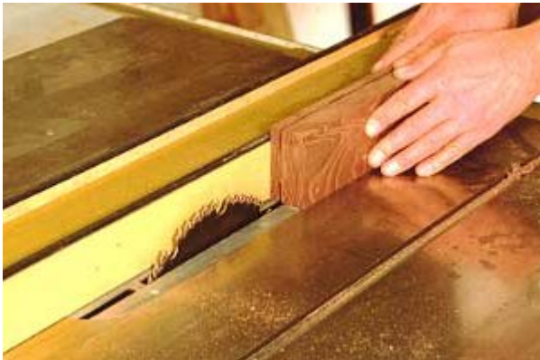
Photo 8- Resaw stock for the slats at the table saw. Make the cuts in stages.
