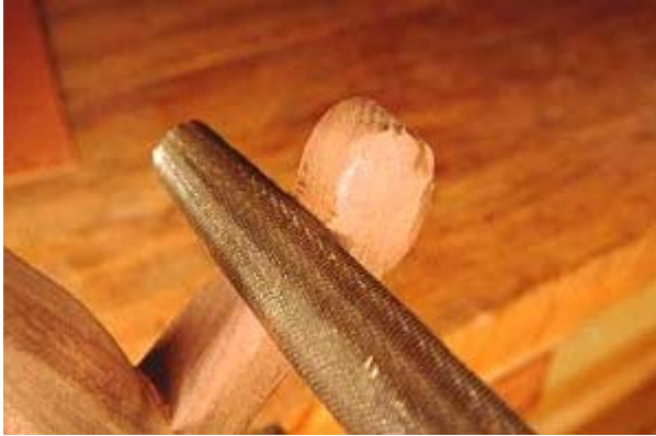
Photo 16- Use a file to get into the corners.
