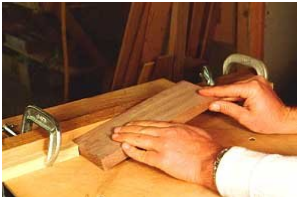
Photo 3- Lift the part off the bit after it touches the far stop.
