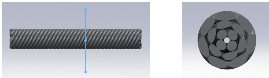
Figure 2.6: Cross section of the modelled yarn.
