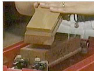
Finish on a 1200 grit water stone
