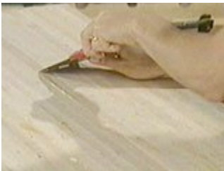
Glue the five larger pieces together and scrape off the excess glue
