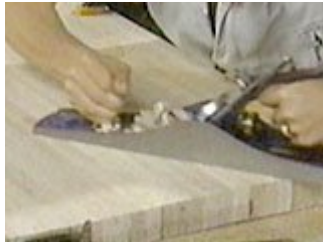
A large plane will provide the flattest surface
