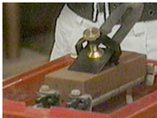
Use a jig to hold the blade fixed while sharpening
