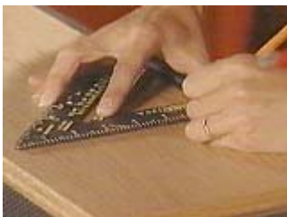
Mark for the peg holes
