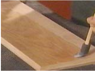
Apply a clear water based finish with a sponge brush
