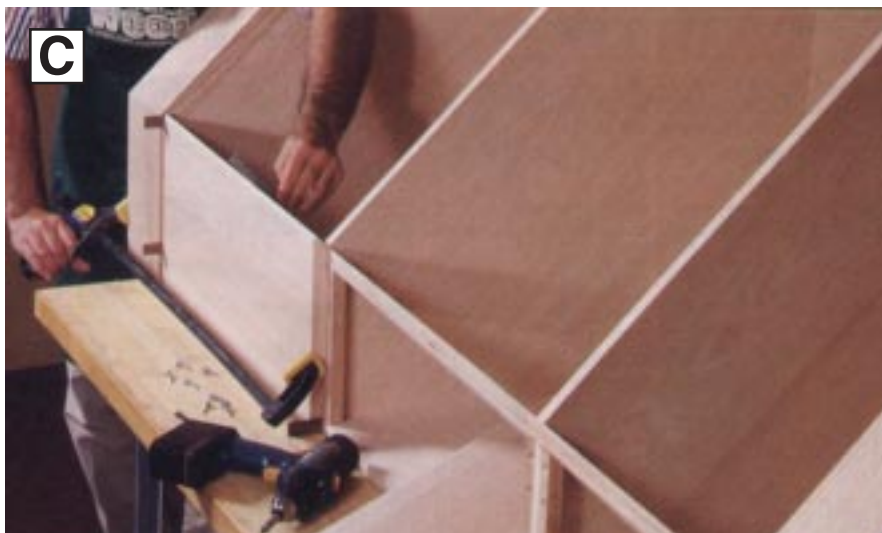
C With the cabinet on its back, use spacers to create equal gaps between the molding and banded side panels.
