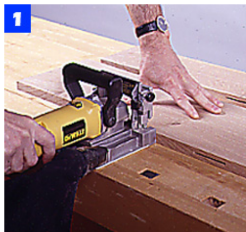
Cut and joint stock for the sides, top, bottom, partition and shelves. Then cut slots in mating edges with a plate joiner.
