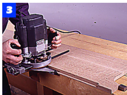
Cut the rabbets for the back panel in the case sides and top using a router with a 3/4-in.-dia. straight bit and edge guide.
