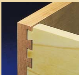
Too Loose. If joint is too loose, increase bit depth. Too Tight. If the joint is too tight, decrease depth.
