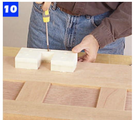
Make the poplar beam-support blocks. Bore pilot holes and screw them to the center of the front and back lower rails.
