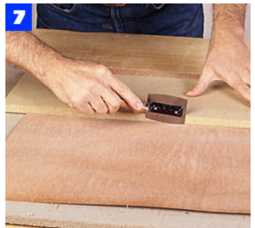
Use a veneer saw and straightedge guide to cut the veneers for the head-board and footboard panels.
