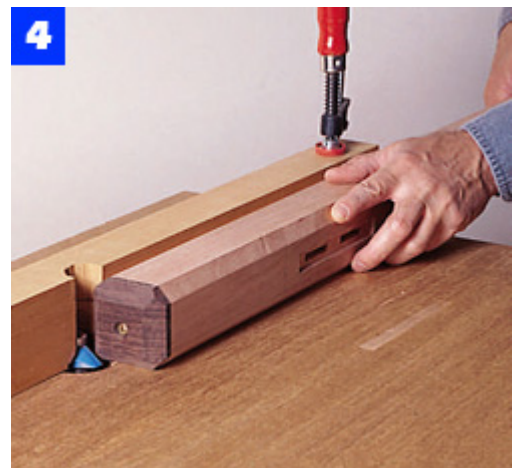
4 Use a chamfer bit in the router table to shape a 3/8-in. chamfer along the long edges of each bedpost.
