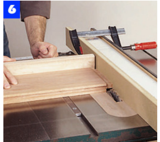
Clamp a scrap board to the rip fence to act as a stop when cutting the tenons on the ends of the rails and stiles.
