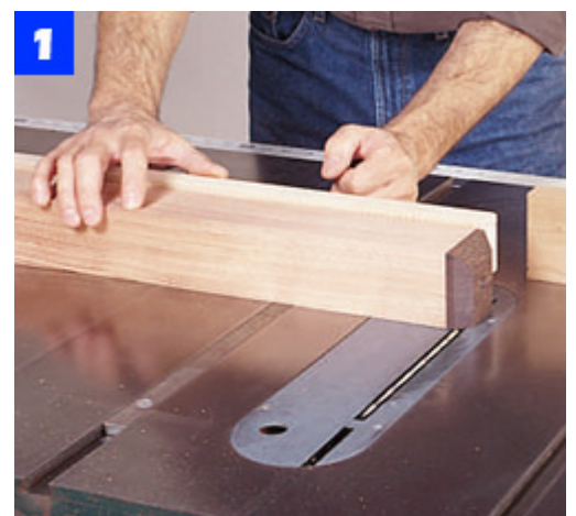
After attaching each wenge foot to a post with glue and a screw, use your table saw to chamfer the edges.
