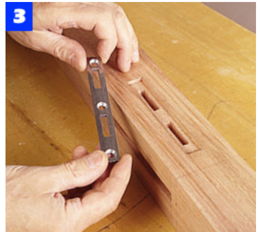
3 Rout the mortises in the posts for the rail-hanger hardware. Then, test the fit and bore screw pilot holes.
