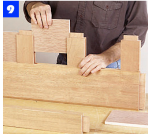
Apply glue to the joints and assemble the stiles and bottom rail. Slide the panels into place and add the top rail.
