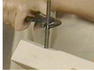
Drive it in with tongue-in-groove pliers
