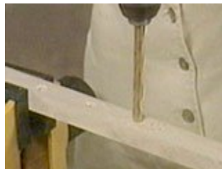
Use a counter sink bit or larger bit to cut a space for the screw
