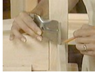
Set the brace on top of the apron to locate the slots
