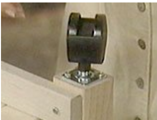
Attach the casters to the bottom of the legs
