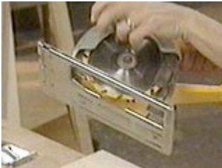
Set the depth of the blade to fit the brace
