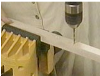
Drill holes every three inches for the screws
