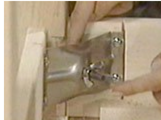
Attach the bracket in place with four screws
