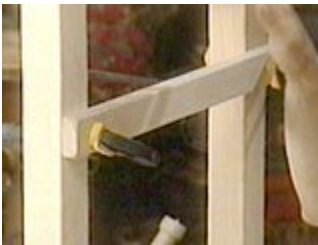
Clamp the shelf supports in place and screw them to the leg
