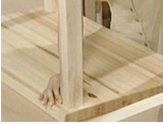
Locate the legs on the bottom of the cutting surface
