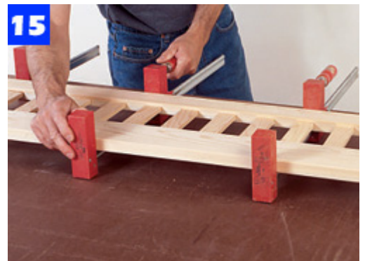
Use three or four clamps to squeeze the front rail assembly, pressing the slats to the bottom of the mortises.
