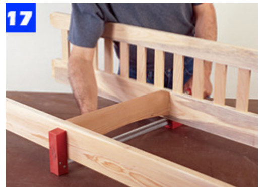
Use a clamp to pull the front rail and back rail assembly tight to the center seat-support rail.
