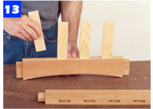
After cutting the curved rail profiles, press the side slats firmly into their mortises. It's not necessary to use glue.
