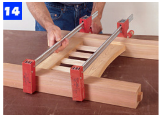
Spread glue in the leg mortises and side rail tenons, and assemble one of the bench sides. Clamp until the glue sets.
