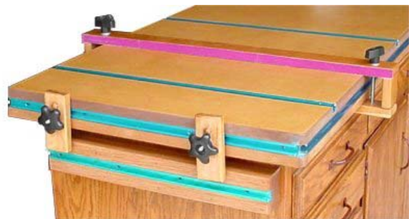
Arranging the jaws for use with the EZ Mount Stop. The purple edge is the 100 grit sandpaper used to make the stop grip the work piece tighter.
