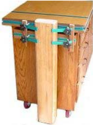
Clamp a large work piece Hold down clamps.
