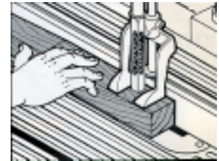
Fig. 3. Cutting mortise in leg (note hold-down).
