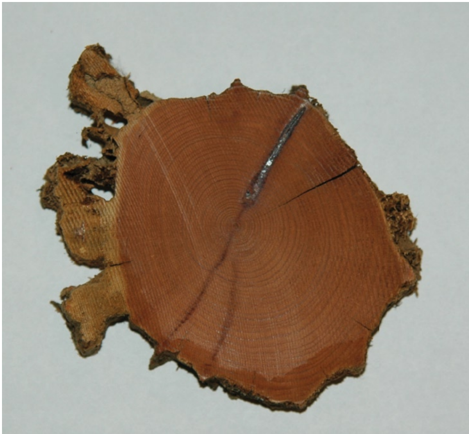
Only the heartwood of naturally-durable species is durable. In this eastern redcedar post, most of the light-colored sapwood has been destroyed by insects and decay. The reddish-colored heartwood portion is still sound.
