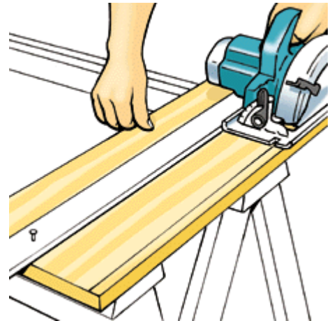
Fig. 3 Use a straight strip as a guide when ripping stock for the four lower shelves to 8 7/8 in. The top shelf remains a full 1 x 10.
