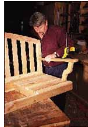
The back of the arm is simply screwed in place through the back stile, while the support is attached to the arm and seat with dowels and polyurethane glue. Notice the foamy squeeze-out of the glue at the joints.
