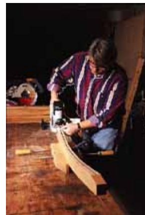
Holding the arched top rail steady was the most difficult part of routing the top groove for the slats. Remember to make the cut in two passes on each side. In this photo you can see that the rail hasn't been cut for length yet, allowing extra support for the router at the beginning and end of the cut.
