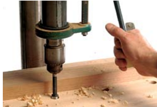
5 Lay out the bench-dog hole locations, and use a drill press and Forstner bit to bore the holes.
