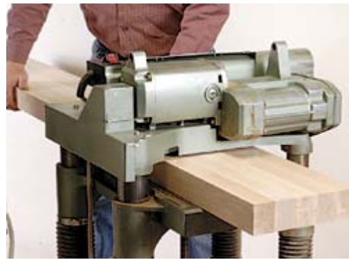
4 After truing one face of each piece with a hand plane, use a thickness planer to mill the opposite sides.
