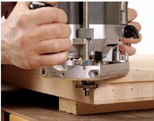
6 Use a slot cutter in your router to shape a spline groove around all edges of the benchtop slab.
