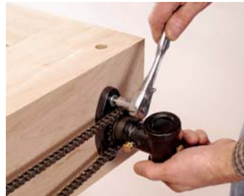
12 After adjusting the chain length, thread end-vice screws in place and attach outer vise collars.
