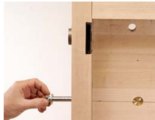
11 Join the end-vice cap to the top with bench bolts. Don't use glue. The top must be free to move.
