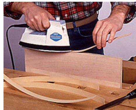
1--Finish the plywood edges with iron-on veneer tape. Set the iron for high heat and press down to activate the hot-melt glue.
