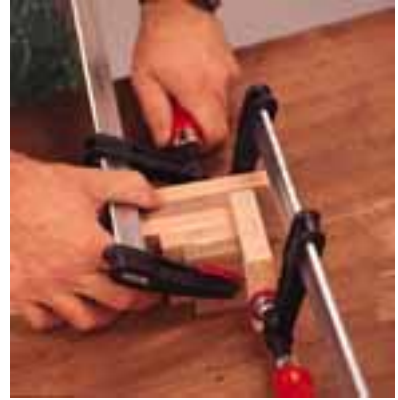
The stop block clamped at the end of the glue-up jig keeps the F4 and F5 pieces level with the top of the G3 piece.
