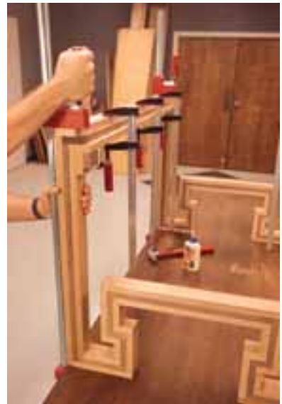
Start by gluing G1 in place, then work your way up. As you can see in the photo, I clamped the entire leg to my assembly bench to make things easier.
