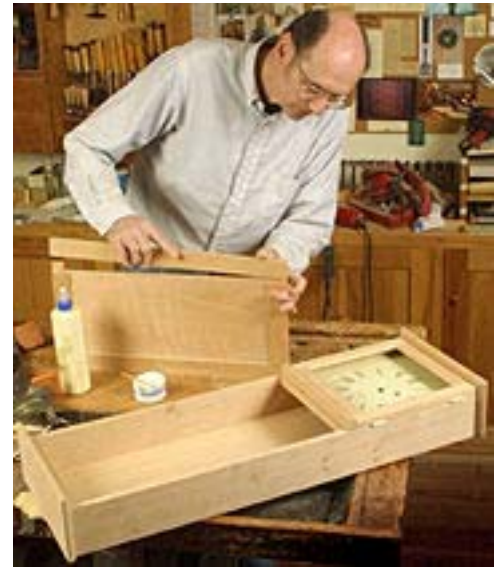
Before applying glue, carefully dry-fit the doors and see that they fit the case.
