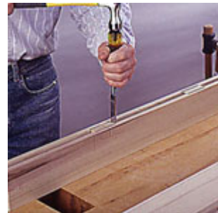
5--After the grooves have been routed, disassemble the headboard and use a sharp chisel to square the rounded ends.
