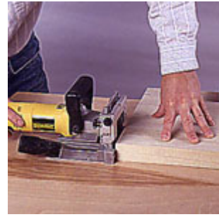
3--To cut the double plate slots, use a flat surface to register the slots on one side. Then, flip over work for remaining slots.
