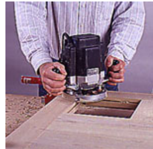
4--Dry assemble the headboard with plates and install clamps. Rout the panel grooves with a piloted slotting bit.
