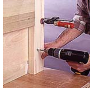
18--Position the headboard and clamp it in place. Bore and countersink pilot holes and screw the headboard to the storage box.
