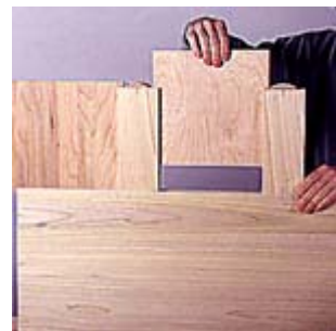
6--Slide the panels into place, and join the top rail to
