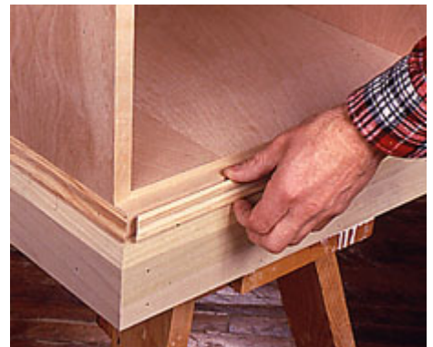
9--Install the baseboard around the desk, then finish the profile by nailing panel molding above the baseboard.
