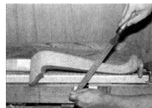
Fig. 10 Chamfer the stock between control lines.
