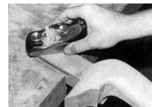
Fig.14 Use a Block Plane to smooth the Leg Posts.
