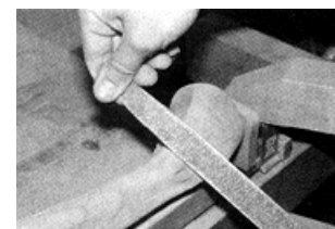
Fig. 11 Feather a flat on the top surface of the Foot.
