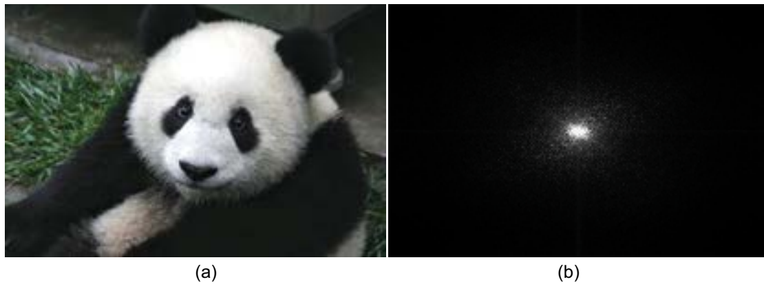
Figure 30 An image of a panda (a), and its power spectrum of the gray level image (b).
