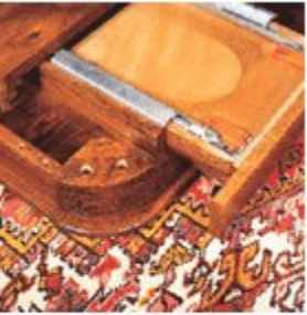
Good hardware is a real workshop timesaver. Turn the table over for a look at the hidden drawer slides?an easy solution for smooth, quiet, self-closing drawers
