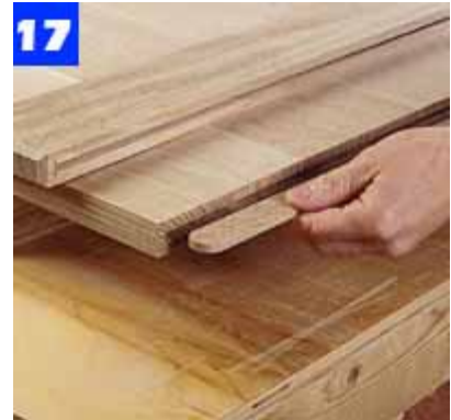
Cut splines for the breadboard-end joints. A 1/2-in. radius on the ends matches the slot profile.
