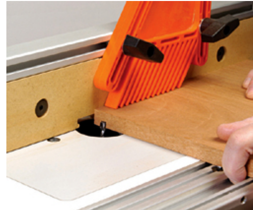
1 Use a 1/4-in. bit and router table to cut the dados in the chest sides for the bottom panel.
