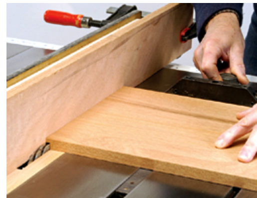
2 Cut the rabbet in the bottom panel with a dado blade. The blade extends into board clamped to fence.
