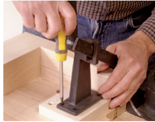
13 Secure a mounting block under the benchtop to support the tilt bracket for the side vise.
