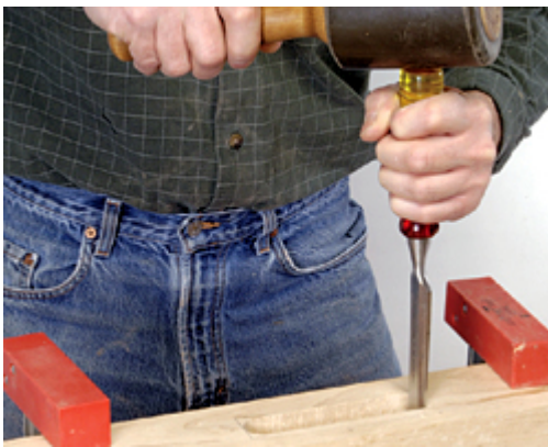
14 Finish the mortises for the stand with a sharp chisel after boring out most of the waste.
