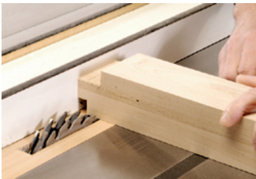
15 Use a dado blade in your table saw to cut the tenons on the leg and stretcher ends.
