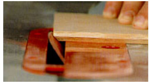
2 TOP CHAMFER • The top is chamfer cut on three edges, and angle cut on the back edge. By moving my rip fence to the left of the blade, my right-tilt saw is able to make the cuts safely, allowing the waste to fall away from the blade.
